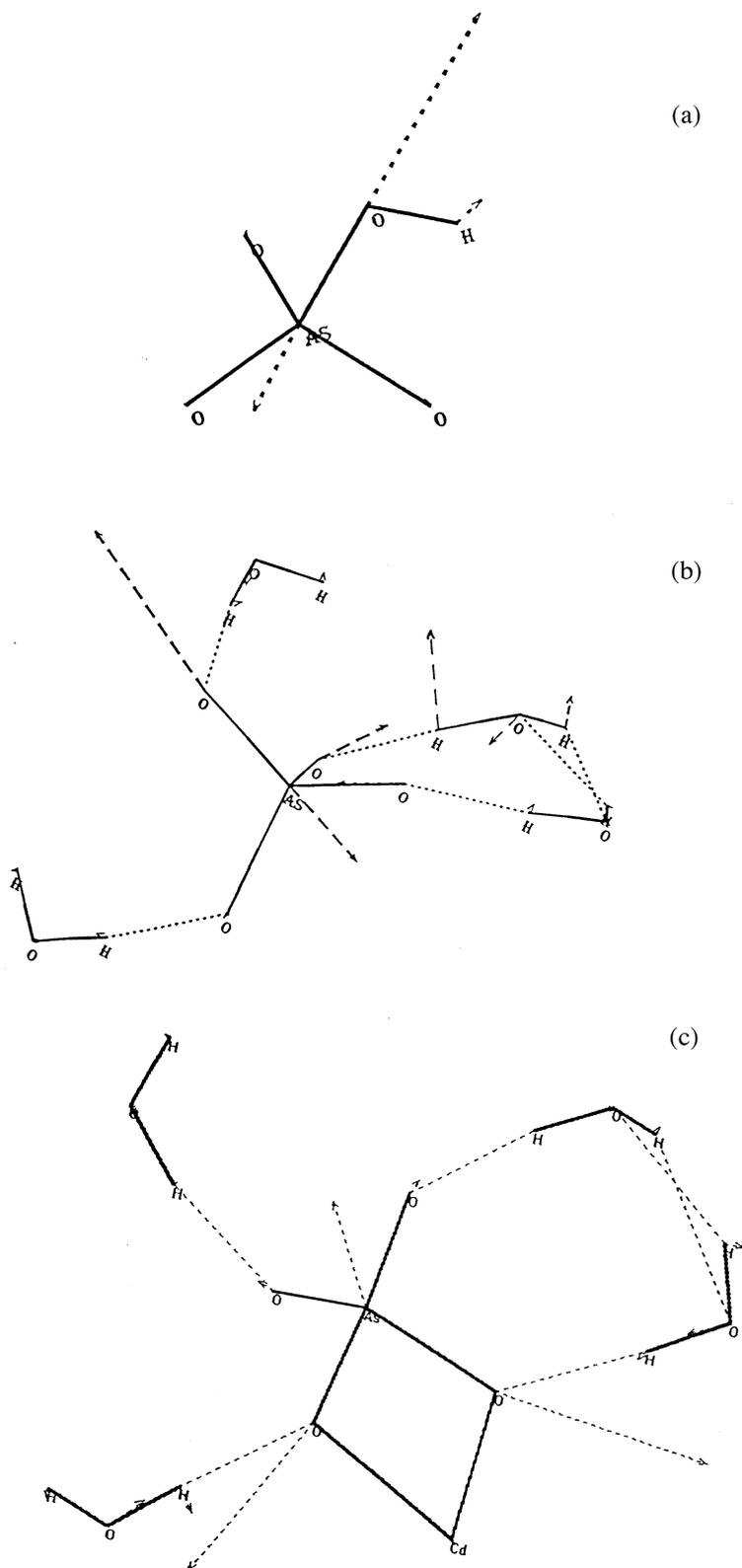
Fig. 1. Examples of  $\text{AsO}_4^{3-}$  molecular clusters used for theoretical vibrational spectra calculations. Solid and dashed lines correspond to interatomic and H-bonds, respectively. Long dashed lines with arrow heads represent symmetric stretching vibrations. The structures are for protonated (a), solvated (b), and metal complexed  $\text{AsO}_4^{3-}$  (c).
