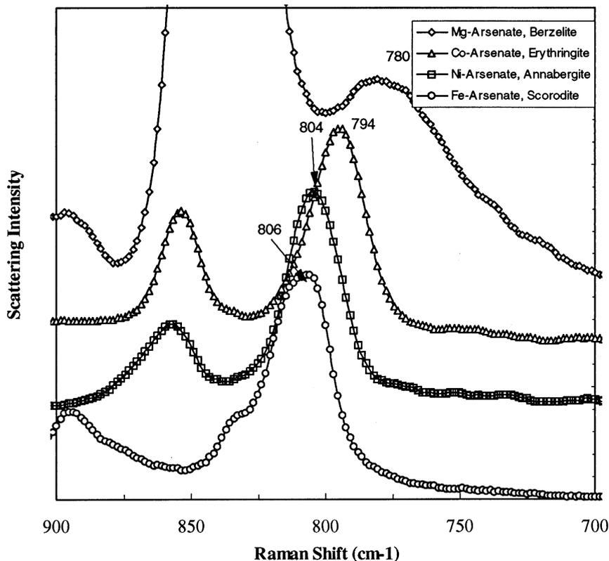
Fig. 6. Raman spectra of As-O stretching vibrations in crystalline metal arsenate salts. For spectral information see Table 4.
