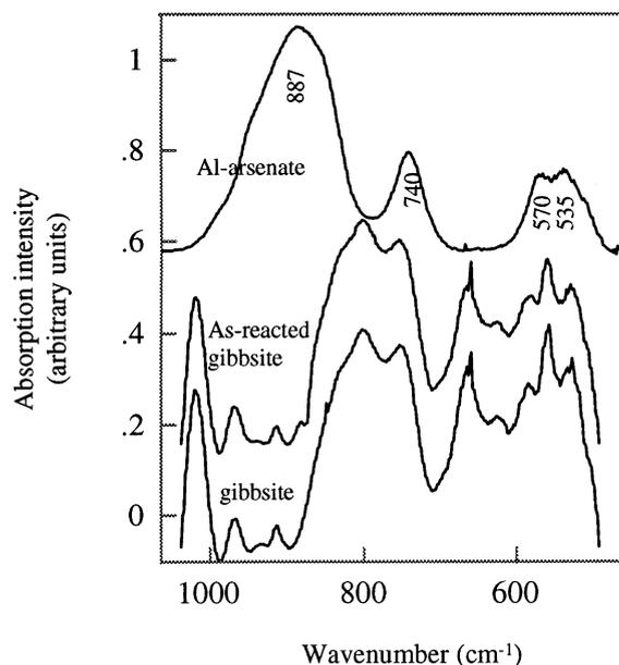
Fig. 8. Diffuse reflectance FTIR spectra of As-O vibrations in Al-arsenate and arsenate reacted gibbsite.
