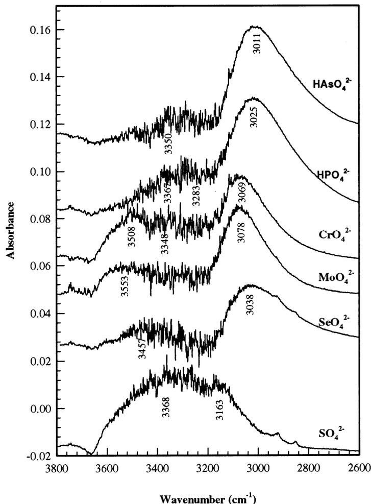
Fig. 3. ATR-FTIR spectra of OH stretching vibrations of H<sub>2</sub>O in the primary oxoanion solvation shell. Oxoanion concentration in aqueous solutions was 10 mM, and the samples were prepared by dissolving Na-salts. Predominant aqueous species of oxoanions are shown with their respective spectra.
