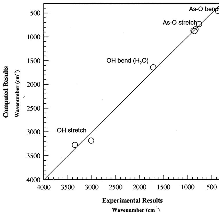
Fig. 2. Comparison of theoretical and experimental vibrational spectra of different  $\text{AsO}_4^{3-}$  species. Refer Table 2 for further details. The points around 3000, 1600, 800, and 400  $\text{cm}^{-1}$  correspond to the OH stretching, OH bending, As-O stretching, and As-O bending vibrations, respectively.
