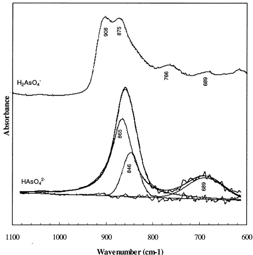
Fig. 5. ATR-FTIR spectra of As-O stretching vibrations of  $\text{HAsO}_4^{2-}$  and  $\text{H}_2\text{AsO}_4^-$ . For spectral assignments refer Table 3.
