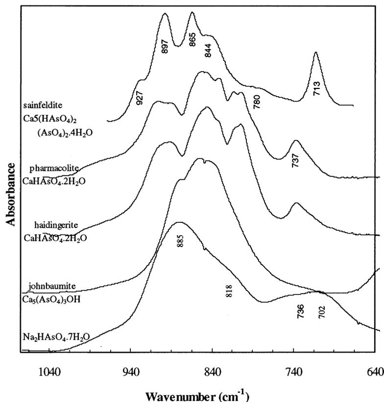
Fig. 7. Diffuse reflectance FTIR spectra of As-O vibrations in crystalline calcium  $\text{AsO}_4^{3-}$  salts.
