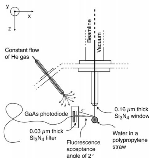
**Figure 1.** Left: The soft X-ray endstation for environmental research (SX-EER). Synchrotron beamline endstation used for O 1s X-ray absorption spectroscopy of liquid water and aqueous solutions. Right: The experimental setup in the sample chamber of SX-EER gives an ambient environment with atmospheric pressure and room temperature.
