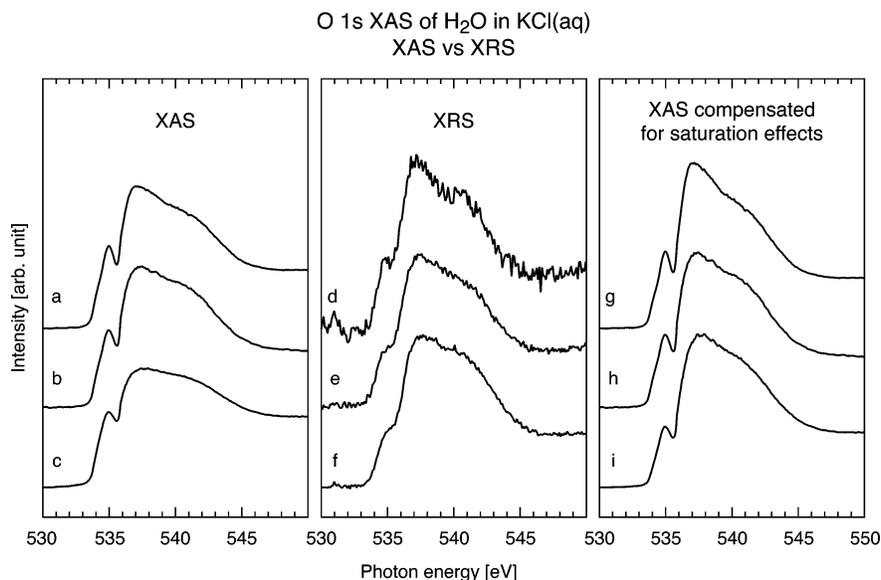
**Figure 3.** O 1s X-ray absorption spectra of (a) 4 m KCl(aq), (b) 1 m KCl(aq), and (c) pure water, as recorded with XAS, (d) 4 m KCl(aq), (e) 1 m KCl(aq), and (f) pure water, as recorded with XRS. The rightmost panel shows corresponding XAS spectra after compensation for saturation: (g) 4 m KCl(aq), (h) 1 m KCl(aq), and (i) pure water.
