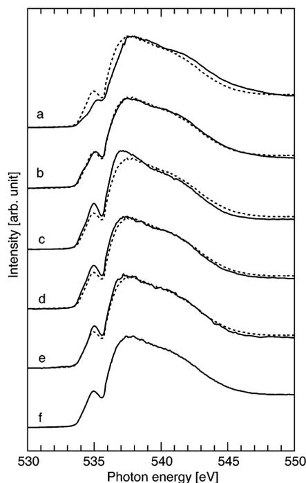
**Figure 5.** O 1s XA of (a) 2.7 m AlCl<sub>3</sub>(aq), (b) 0.9 m AlCl<sub>3</sub>(aq), (c) 4.0 m KCl(aq), (d) 1.0 m KCl(aq), (e) 1.0 m NaCl(aq), and (f) pure water. The 1.0 m NaCl(aq) and 1.0 m KCl(aq) spectra show small changes compared to the pure water spectrum (dotted), while the 4.0 m KCl(aq) spectrum shows larger changes. The 0.9 m AlCl<sub>3</sub>(aq) spectrum shows a very small change compared to pure water (dotted), despite the fact that Al<sup>3+</sup> is a strongly hydrated cation.
